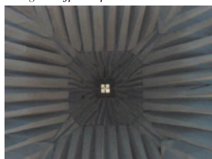
▲ Fig. 2 Shaping from square to octagonal cross-section at the feed.
