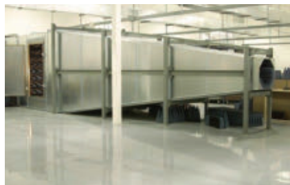
▲ Fig. 1 A typical tapered anechoic chamber.
